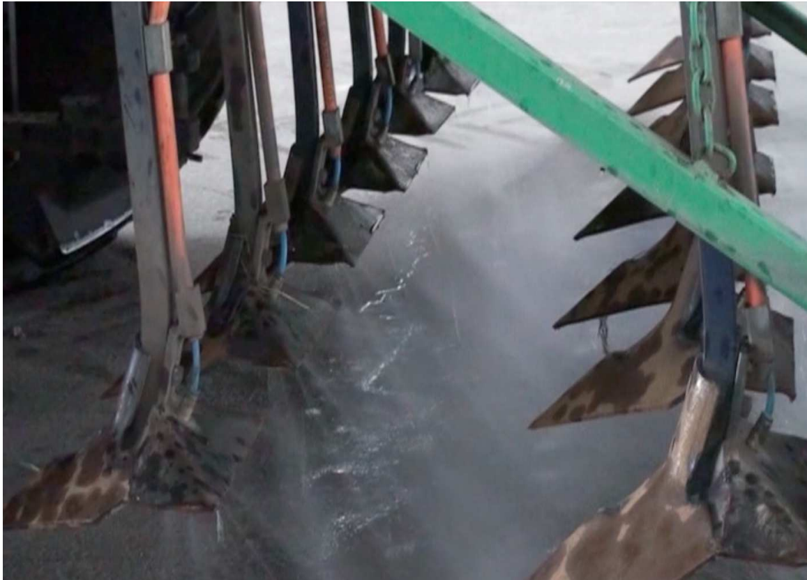
Figure 3 The closely spaced tynes, spraying water, in a demonstration of how the chemical is evenly sprayed into the soil
