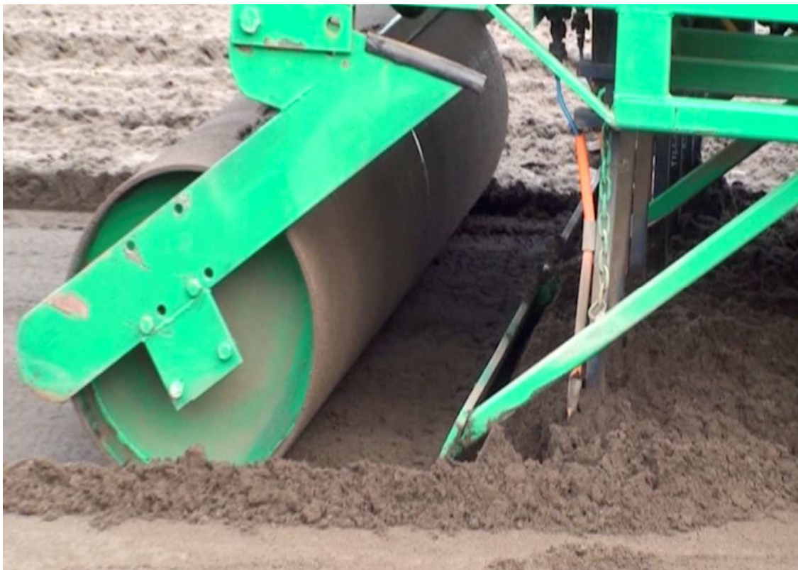
Figure 2 Behind the buried tynes that create space for the spray nozzles to apply the chemical, a flat bar levels the soil before the heavy roller seals the soil to prevent loss of gasses.
